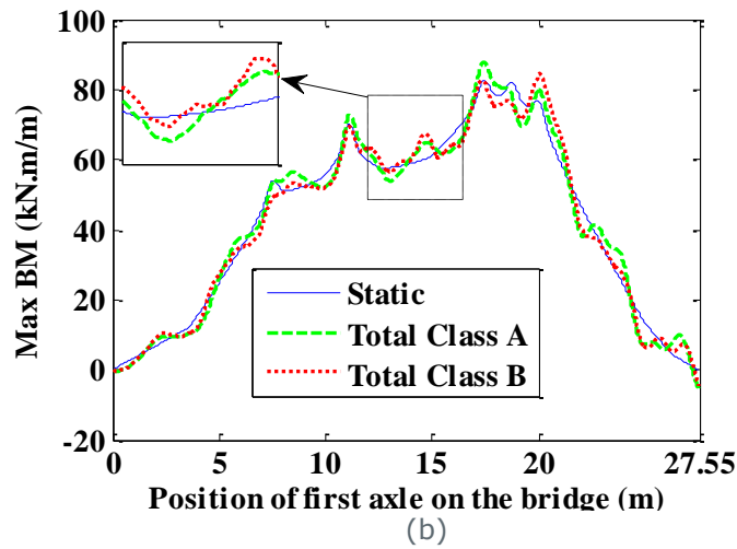
Figure 28. Static and total Bending Moments (BM) (kN.m/m) for class 'A' and class 'B' road profiles at the node holding maximum static value (i.e. node no. 18 in section 'A-A') versus position of first axle of Case_0_b truck travelling on the bridge at (a) critical speed, (b) 60 km/h
