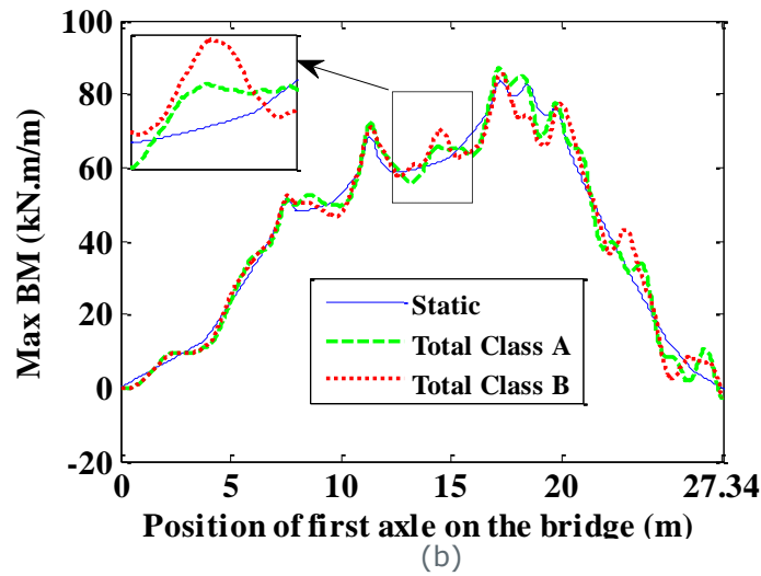
Figure 40. Static and total Bending Moments (BM) (kN.m/m) for class 'A' and class 'B' road profiles at the node holding maximum static value (i.e. node no. 18 in section 'A-A') versus position of first axle of Case_2 truck travelling on the bridge at (a) critical speed, (b) 60 km/h
