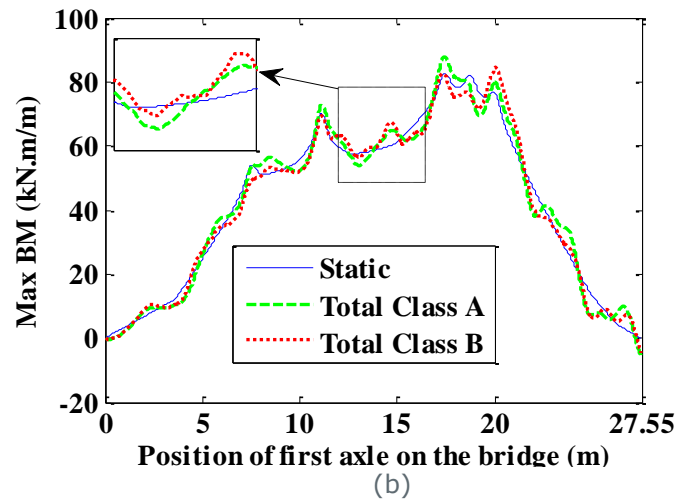
Figure 28. Static and total Bending Moments (BM) (kN.m/m) for class 'A' and class 'B' road profiles at the node holding maximum static value (i.e. node no. 18 in section 'A-A') versus position of first axle of Case_0_b truck travelling on the bridge at (a) critical speed, (b) 60 km/h
