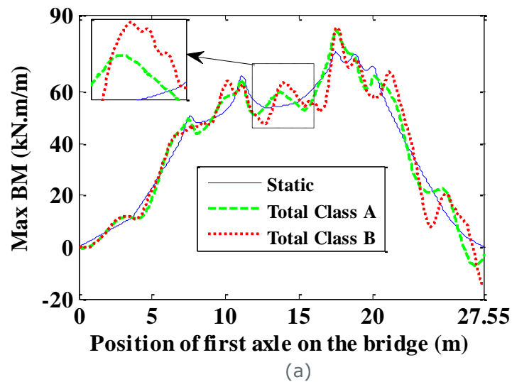
Figure 33. Static moment at section 'A-A' (kN.m/m) of Case_0_d truck
