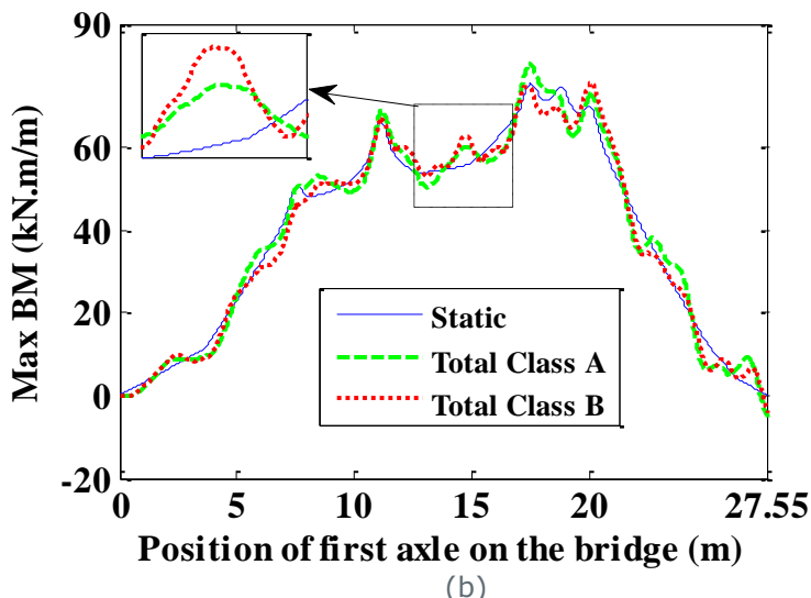
Figure 34. Static and total Bending Moments (BM) (kN.m/m) for class 'A' and class 'B' road profiles at the node holding maximum static value (i.e. node no. 17 in section 'A-A') versus position of first axle of Case_0_d truck travelling on the bridge at (a) critical speed, (b) 60 km/h
