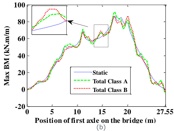
Figure 37. Static and total Bending Moments (BM) (kN.m/m) for class 'A' and class 'B' road profiles at the node holding maximum static value (i.e. node no. 18 in section 'A-A') versus position of first axle of Case_1 truck travelling on the bridge at (a) critical speed, (b) 60 km/h
