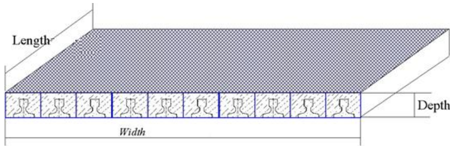
Figure 14. Cross-section of Inverted T-beam bridge model.
