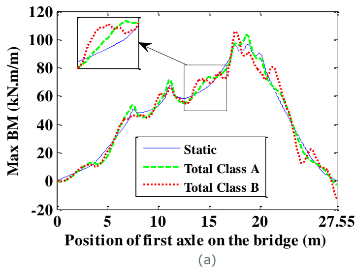
Figure 30. Static moment at section 'A-A' (kN.m/m) of Case_0_c truck
