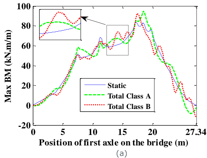
Figure 39. Static moment at section 'A-A' (kN.m/m) of Case_2 truck
