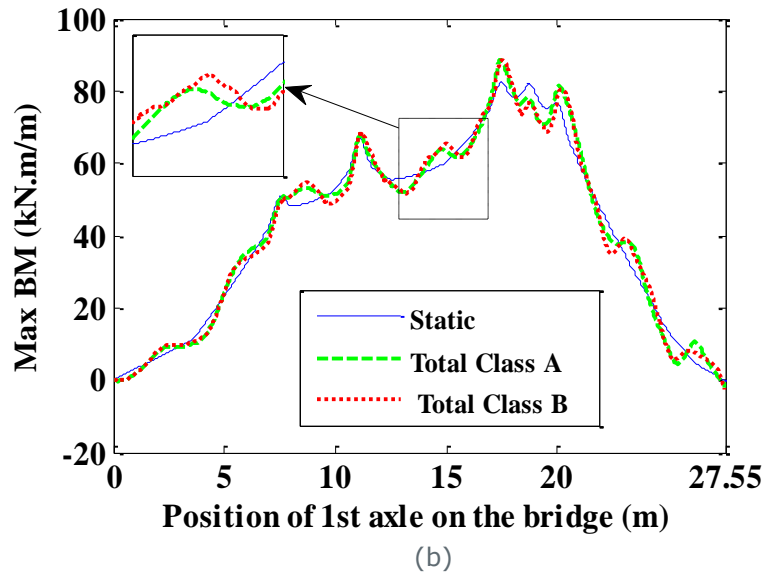
Figure 25. Static and total Bending Moments (BM) (kN.m/m) for class 'A' and class 'B' road profiles at the node holding maximum static value (i.e. node no. 18 in section 'A-A') versus position of first axle of Case_0_a truck travelling on the bridge at (a) critical speed, (b) 60 km/h
