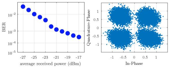
Figure 3. 3 BER as a function of the received power (a) and measured constellation diagram for a received power of -22dBm (b).
