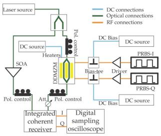
Figure 2. Experimental setup employed for QPSK signal characterization.
