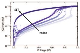
Fig. 8. Current of the PCM versus Bit Line voltage for several intermediate states, allowing the extraction of the conduction parameters. Dots are measurements, lines are simulations. The only parameter varying is the amorphous thickness *u<sub>a</sub>*.
