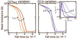
Fig. 13. Impact of the variation of the parameters  $\tau_{OHT}$  and b on the growth speed. (a)  $\tau_{OHT}$  acts on the mean crystallization time; (b) b increases the growth speed for low amorphous fraction (inset), so enhances the positive feedback on the Rampdown SET crystallization speed.
