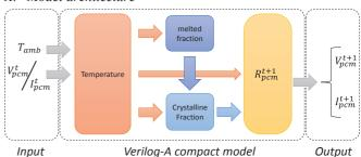
Fig. 1. Modeling flow block diagram
