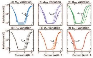
Fig. 12. Impact of the static parameters on the RESET-SET-RESET characteristics. (a)  $R_{c\theta}$  rules the conduction in the SET regime; (b)  $A_{kPF}$  impacts the RESET resistance; (c)  $R_{thc}$  increases the internal temperature, which is mostly seeable in the melting phase; (d) The average melting temperature  $T_m$  impacts the SET to RESET transition current; (e)  $\sigma_m$  changes SET to RESET transition spread; (f)  $\tau_{\theta LT}$  deals with RESET to SET transition.
