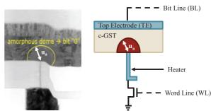
Fig. 5. TEM cross section of the test structure on the left hand side and equivalent schematics on the right hand side.
