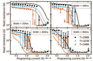
Fig. 11. SET Low characteristics: Transition from RESET to SET using low current density for four pulse widths under three operating temperatures. Dots are measurements, lines are simulations. Error bars are obtained by repeating three times the exact same set of measurements. The dynamics is hard to fit with the same model card as the Rampdown SET, as tradeoff has to be found to fit both characteristics.
