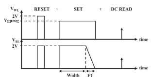
Fig. 7. Detail of the pulse sequence applied to get one measurement. WL programming voltage (Vgprog), pulse width (Width) and fall time (FT) are the programming variables. Reading BL voltage is set at 0.1V. Delays between pulses are fixed to avoid drift effect issue
