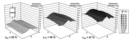
Fig. 11. Evolution of experimental volumetric dilatation extrapolated by projection in the specimen cross-section for composite A.
