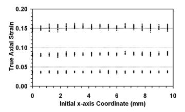
Fig. 3. Dispersion of true axial strain  $\varepsilon_{xx}$  values measured in 400 points on front side of material B for three different loading levels.
