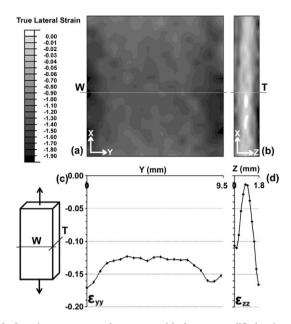
Fig. 8. Local transverse strains measured in impact-modified polypropylene B for  $\varepsilon_{xx} = 49\%$  ((a) front transverse strain field  $\varepsilon_{yy}$ ; (b) lateral transverse strain field  $\varepsilon_{zz}$ ; (c) local front transverse strains on line W; (d) local lateral transverse strains on line T).
