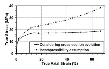
Fig. 7. Influence of incompressibility assumption on experimental stress-strain curve for composite B.
