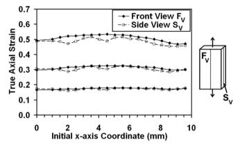
Fig. 4. True axial strain  $\varepsilon_{xx}$  measured from front and lateral pattern correlations for three loading levels in composite B.
