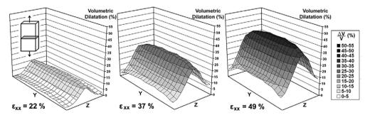
Fig. 10. Evolution of experimental volumetric dilatation extrapolated by projection in the specimen cross-section for composite B.
