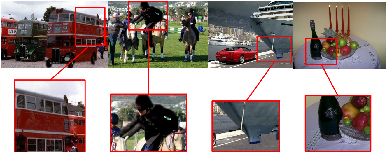
Fig. 8: Illustration of artifacts arising from enlargement augmentation. In the enlargement data augmentation, an instance is cut out of the image, up-scaled by a small factor and placed back at the same location. This approach leads to blending artefacts. Modified images are given in the top row. Zoomed parts of the images centered on blending artifacts are presented in the bottom line.
