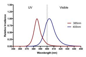
**Figure 7.** The spectral outputs of the experimental sources. The spectral output of the 385 nm and 405 nm Loctite LED sources used in all the studies. The full width at half maximum (FWHM) of the sources were 7 nm and 10 nm respectively. Spectra (350–450 nm) were measured with a Bentham spectroradiometer.
