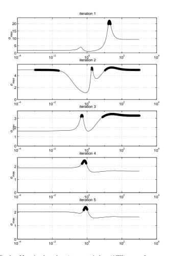
Fig. 1. Max singular values (transport airplane 'AC8') versus frequency - first 5 iterations - '\*' selected frequencies
