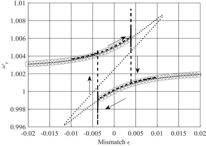
Fig. 6. Comparison of calculated solution of (13) (dots and circles, as in Fig. 5) and transient simulation results (dashed lines) obtained by slowly sweeping  $\varepsilon$  up and down in a Simulink model of (1), with  $Q = 1000$  and  $\kappa = 5 \cdot 10^{-3}$ .
