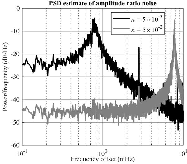
Fig. 3. Spectrum of amplitude ratio fluctuations when the system is subject to independent white noise perturbations  $n_x$  and  $n_y$ . Simulation parameters are  $\omega=1$ ,  $F=1$ ,  $Q=1000$ ,  $\varepsilon=0$ .
