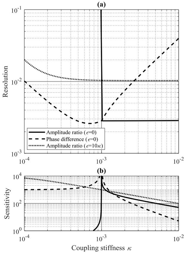
Fig. 7. Resolution (a) and sensitivity (b) of the amplitude ratio (full lines), phase difference (dashed lines) output metrics vs. coupling coefficient  $\kappa$ , resulting from the analytical solution of (17). The dotted curves are obtained for the amplitude ratio, when  $\varepsilon=10\times\kappa$ . The quality factor is  $Q=1000$ , and the resolution is calculated for  $N=1$ , and  $\Delta f=1$ .
