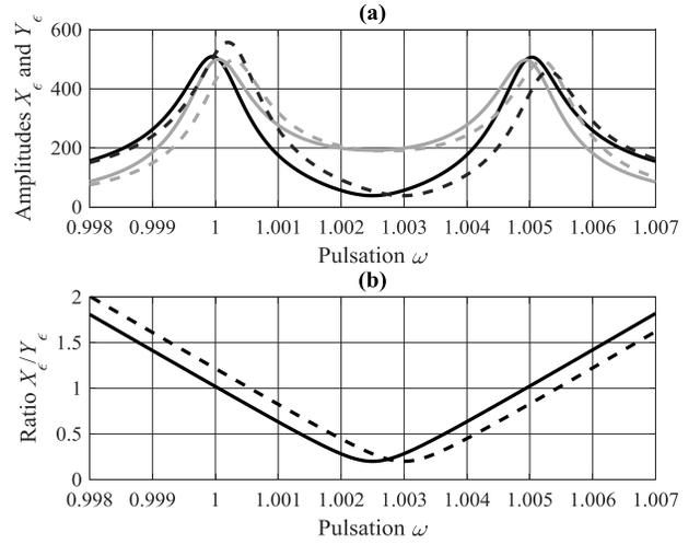
Fig. 2. Amplitude responses (a) of the resonators ( $X = \text{black}$ ,  $Y = \text{grey}$ ) and amplitude ratio (b) for  $\varepsilon=0$  (full lines) and  $\varepsilon=10^{-3}$  (dashed lines). The system parameters are  $F=1$ ,  $Q=1000$ ,  $\kappa=5.10^{-3}$ .
