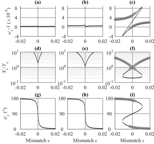
Fig. 5. Steady-state characteristics of the oscillator versus mismatch  $\varepsilon$  for  $\kappa Q = 0.5$  (a,d,g),  $\kappa Q = 1$  (b,e,h) and  $\kappa Q = 5$  (c,f,i). The quality factor is  $Q = 1000$ . For  $\kappa Q = 5$ , the grey circles indicate the stable solutions.
