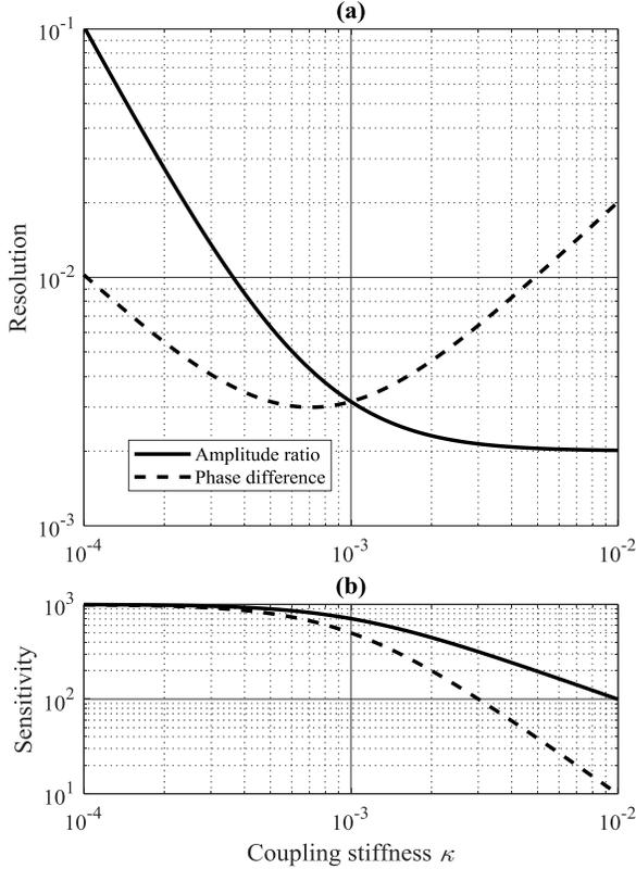
Fig. 4. Resolution (a), and sensitivity (b) of the amplitude ratio (full lines) and phase difference (dashed lines) output metrics vs. coupling coefficient  $\kappa$ , resulting from the analytical solution of (7). Calculation parameters are  $\omega=1$ ,  $Q=1000$ , and  $\varepsilon=0$ . The resolution is calculated for  $N=1$ , and  $\Delta f=1$ .
