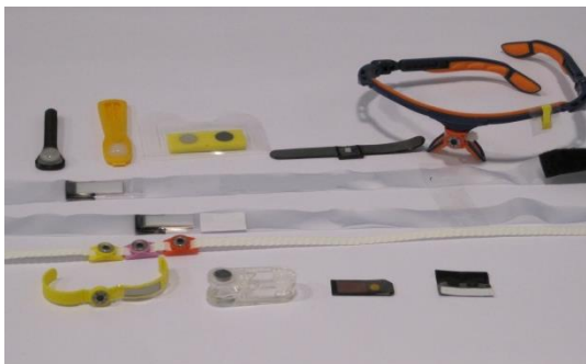
Figure 1. Photo of the different types of dosimeters provided by the participants for the IC2014 eye .
