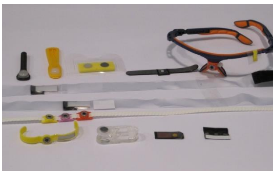
Figure 1. Photo of the different types of dosimeters provided by the participants for the IC2014 eye .
