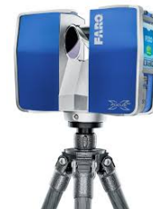
Figure 2. Characteristics and photograph of the Faro ® Focus 3D X330 TLS.
