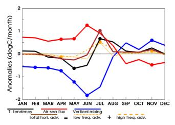
Figure 7. Cold ACT events anomalies to the mean annual cycle of the mixed-layer heat budget terms (in °C/month) averaged in the central box [15°W-6°W, 4°S-1°N]. Dots indicate the significance at the 90% confidence level.
