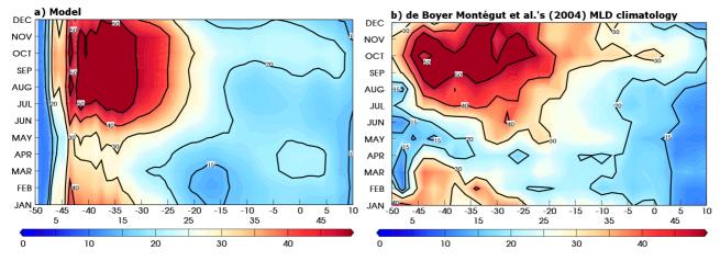
Figure 4. Same as Figure 2 for a) the simulated MLDs and b) de Boyer Montégut et al.'s (2004) MLDs climatology in m (isoline at 15 m and 20 m then every 10 m).
