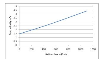
Figure 2: Droplet velocity vs helium flow with the venturi system.
