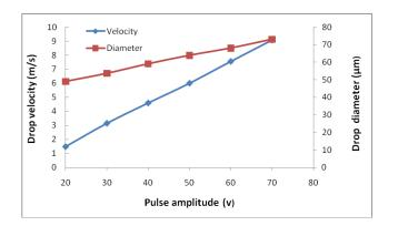
Figure 3: Drop velocity and diameter as a function of piezoelectric excitation voltage for an ink-jet  $50\mu m$  dia. nozzle.
