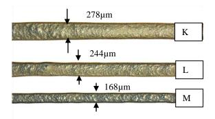
Figure 4: Comparison between the 3 methods. ZnO nanoparticles deposited on Silicon substrate at  $65^{\circ}$ C; nozzle diameter 50µm; more spacing between two droplets: 50µm; contact angle  $17^{\circ}$ .
