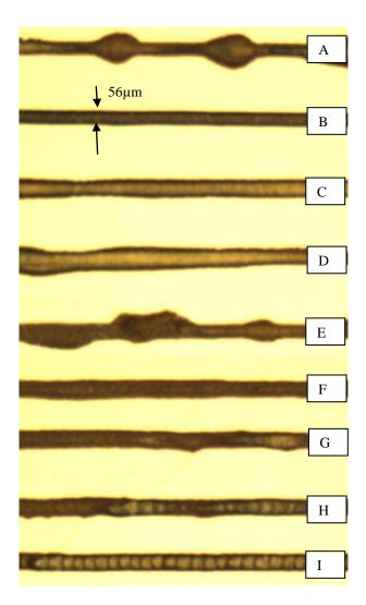
Figure 1: Optical picture of ZnO nanoparticles deposited on gold layer at different temperatures. Contact angle  $40^{\circ}$ ; diameter of the nozzle 50µm; distance between two droplets 50µm.
