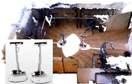
Figure 1. An example of 3D indoor mapping with two simultaneously operating mobile RGB-D sensor platforms [4].
