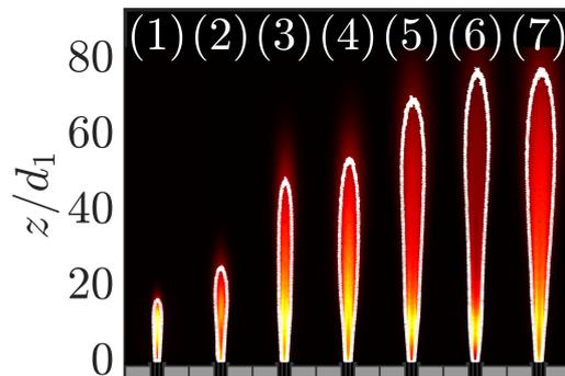
Figure 2: OH\* intensity distribution of selected flames from dataset D2 in Tab. 1 and increasing  $\Phi_m$  values. Numbers refer to Fig. 4b. White contours indicate the Otsu threshold used to determine  $L_S$ .
