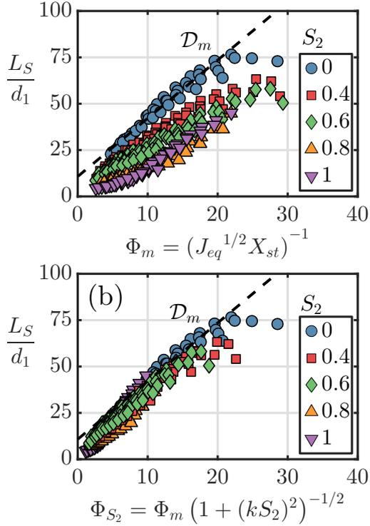
Figure 6: Flame lengths from dataset D4 in Tab. 1. Top : Original scaling  $\Phi_m$  from [8, 14]. Bottom : New model  $\Phi_{S_2}$  accounting for the swirl level  $S_2$  in the outer stream.  $\mathcal{D}_m$  : Eq. (4).
