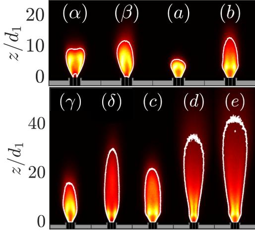
Figure 3: OH\* intensity distribution of selected flames from datasets D5 and D6 in Tab. 1 with high annular swirl levels  $S_2$ . Latin letters refer to data shown in Fig. 7. Greek letters make references to data shown in Fig. 8. White contours indicate the Otsu threshold used to determine  $L_S$ .
