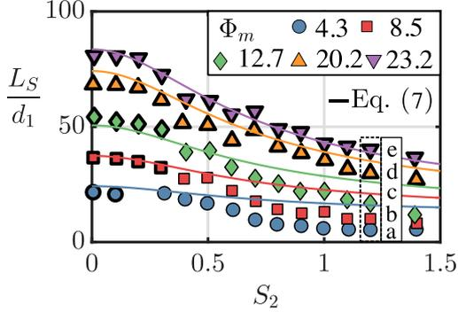
Figure 7: Flame lengths from the dataset D5 in Tab. 1 as a function of the swirl number  $S_2$  for different values of mixing parameter  $\Phi_m$ . Solid lines correspond to predictions from Eq. (7). Symbols with thickened contour designate flames in jet-like regime according to [30].
