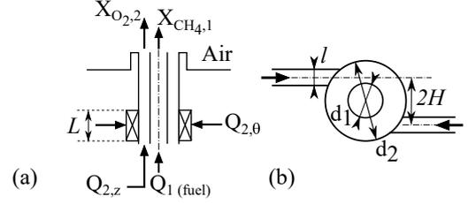
Figure 1: Sketch of the coaxial injector. (a) Axial cut. (b) Transverse cut through the swirler.
