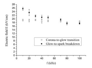
Fig. 2. Transition electric fields (Corona-to-glow and Glow-to-spark) as a function of repetition frequency. Air velocity is kept constant at 3.4 m/s.
