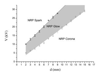
Fig. 1. Domain of existence of the NRP glow regime for a given set of parameters (v = 3.4 m/s, f = 10 kHz).
