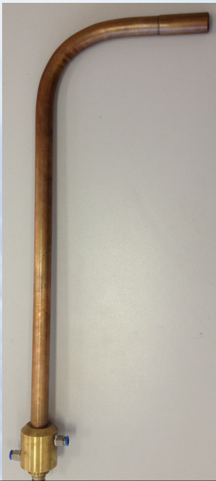
Sample support with water cooling system and probing access
