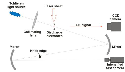
Figure 1. Scheme of experimental setup. Focal length of the lens is 1 m. Spherical mirrors have 2 m focal distance.
