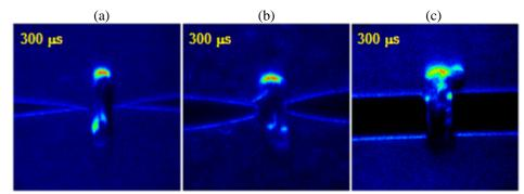
Figure 4. Schlieren images obtained for a single nanosecond spark in air at P=1 atm, U=36 kV for different electrode systems: a) conic stainless steel pin with 30-µm radius of curvature tips; b) paraboloid tungsten pins with tapered 150-µm tip radius; c) cylindrical tungsten electrodes of diameter 2 mm. The distance between the electrodes is 1 mm. The horizontal knife edge cuts 90 % of the light.
