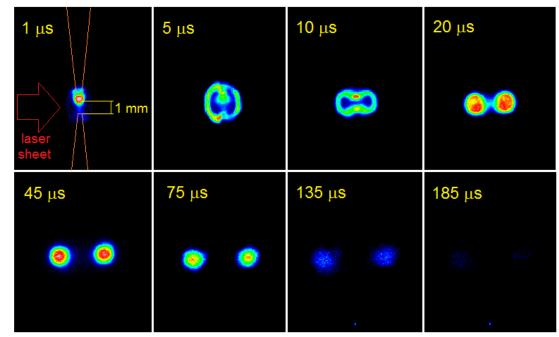
Figure 6. Phase-locked OH LIF images obtained in afterglow of a single nanosecond spark in ambient humid air at P=1 bar. The discharge was initiated in pin-to-pin geometry at U=+36 kV, 10 ns pulse duration. The gap between the pins is 1 mm.
