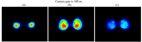
Figure 7. Phase-locked LIF images obtained in afterglow of a single nanosecond spark (at 75 μs) in ambient humid air at P=1 bar. The discharge was initiated in pin-to-pin geometry at U=+36 kV, 10 ns pulse duration. Camera gate is 100 ns. a) 1 mm between the pins, OH LIF; b) 2 mm between the pins, OH LIF; c) 2 mm between the pins, NO LIF;
