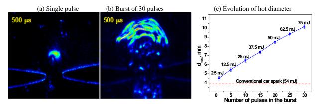
Figure 5. Schlieren results obtained at 500  $\mu$ s after the discharge in air at *P*=1 atm, *U*=28 kV and 1 mm distance between the electrodes; a) single pulse; b) burst of 30 pulses at *f*=70 kHz; c) Dependence of the hot gas core size  $d_{max}$  at 500  $\mu$ s on the number of pulses at 70 kHz. The red dashed line represents the expansion size for the conventional automotive spark.
