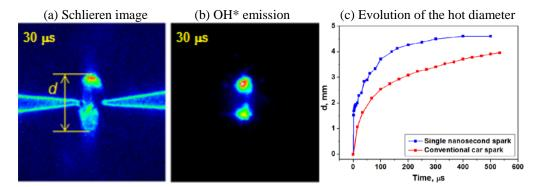
Figure 3. Comparison of a) Schlieren image and b) distribution of spontaneous OH\* emission (308 nm) at 30  $\mu$ s after a single nanosecond spark in air at *P*=1 atm, with a 10 ns pulse of amplitude *U*=36 kV,  $\epsilon$ =6 mJ; c) Evolution of the hot core diameter *d*; Nanosecond spark (blue curve): *U*=36 kV, 10 ns pulse, deposited energy:  $\epsilon$ =6 mJ. Conventional automotive spark (red curve):  $\epsilon$ =55 mJ. Distance between pins: 1 mm.
