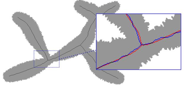
Figure 13: Accuracy of AOF-based skeleton for synthetic shape n°5 at noise level  $\eta = 3$ . In the zoomed part, blue pixels belong to the computed skeleton, whereas red pixels belong to the ground truth skeleton
