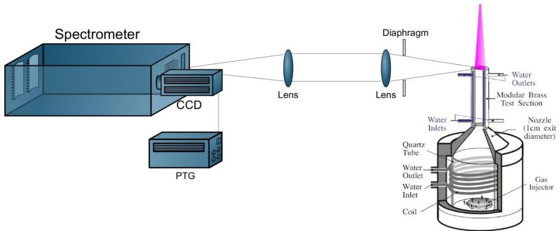
**Figure 3: Experimental setup used for emission spectroscopy**
