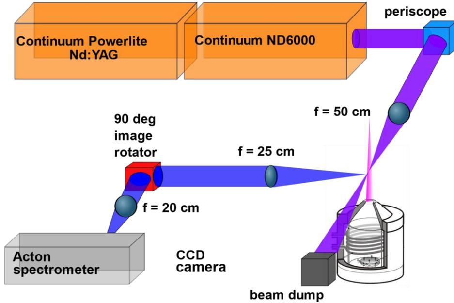
**Figure 4: Experimental setup for Raman UV scattering measurements.** A periscope consisting of two quartz prisms allows to adjust the height and direction of the laser beam. The 90° image rotator serves to horizontally align the laser beam with the spectrometer entrance slit.
