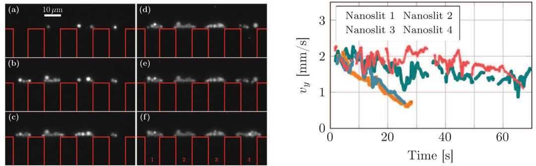
**Figure 4.** Left: image of the development of four adjacent polymersome clogs at the entrance of pores. Red lines delimit the nanoslits. For (a) to (f) the corresponding times are  $t = 0, 14, 28, 42, 56, 70$  s. Right: Sliding average of instantaneous longitudinal velocities of multiple polymersomes flowing through each nanoslit versus time. Nanoslits numbers correspond to numbers written on the left figure (f).
