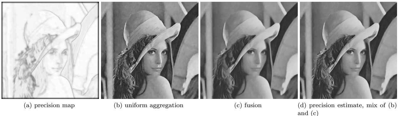
Fig. 15: The inverse of the diagonal of the covariance matrix gives us the precision of the marginal of each pixel. This is a basic estimate of how confident the model is for each pixel. This enables to compute the precision estimate, which tries to keep the best of both worlds.
