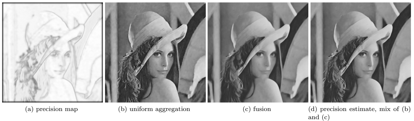
Fig. 14: The inverse of the diagonal of the covariance matrix gives us the precision of the marginal of each pixel. This is a basic estimate of how confident the model is for each pixel. This enables to compute the precision estimate, which tries to keep the best of both worlds.
