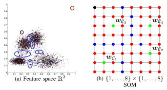
Fig. 7. Simple simulation of Fig. 6 with its equivalent in the SOM geometry. Green bullets on the map correspond to the winning neurons  $w_{\mathcal{C}_k}$  of the class centers  $\mathcal{C}_k$ , blue bullets, on the map in (b), correspond to the location of the neurons that are located in between classes in  $\mathbb{R}^2$ . The black neuron at the top left of the map corresponds to the winning neuron of the sample rounded with a brown ellipse at location (0.2, 0.6).
