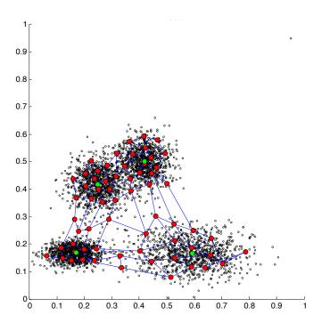
Fig. 6. Simple simulation of a 4-class manifold with an outlier. Samples of the data set in  $\mathbb{R}^2$  are shown with black crosses, the red bullets characterize the locations of the neurons of Kohonen's map. Blue lines show the SOM projected in the feature space. The 4 green bullets characterise the K-means class centers
