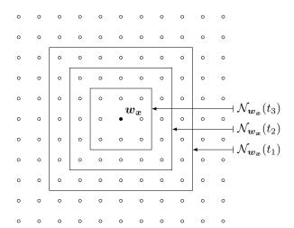
Fig. 1. A schematic view of a  $11 \times 11$  Kohonen's Self Organizing Map. Several topological neighborhood  $\mathcal{N}_{\boldsymbol{w_x}}(t_i)$  of the winning neuron  $\boldsymbol{w_x}$  are drawn. The size is decreasing with the number of iterations  $(t_1 < t_2 < t_3)$  during the training phase, according to (17).
