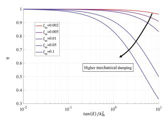
**Fig. 9.** Normalized harvested power boundary  $\eta$  at resonance ( $\Omega_m = 1$ ) with various dielectric losses, coupling, and mechanical damping.
