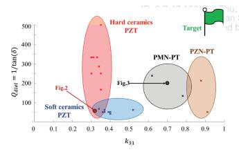
Fig. 4. Coupling  $k_{31}$  and loss tangent  $\tan(\delta)$  of various materials exhibiting piezoelectric properties characterized under small electric fields, with data from Refs. [16, 20–25].
