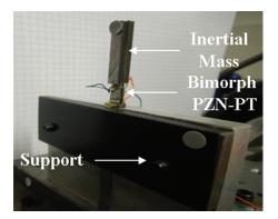
Fig. 12. Piezoelectric harvester made with two plates of PZN-PT.
