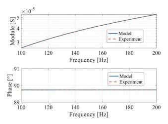
Fig. 3. Experimental admittance analysis of a PMN-PT material and fitted analytical model.
