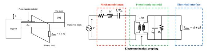
Fig. 7. Piezoelectric energy harvester representation and its associated electrical equivalent model.
