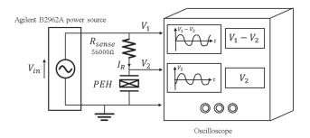
**Fig. 5.** Experimental setup for exhibiting the non-linear behavior of the dielectric losses.
