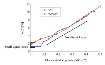
Fig. 6. Evolution of  $\tan(\delta)$  as a function of the AC electric field amplitude applied on the piezoelectric materials.
