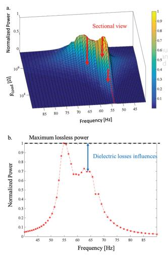
Fig. 16. Experimental harvested power (a) in the  $(R_{\text{load}}, f)$  plane and (b) as a function of the frequency f with an optimal  $R_{\text{load}}$  maximizing the harvested power, with  $\tan(\delta) \approx 10\%$  and  $\gamma = 0.1$  G.
