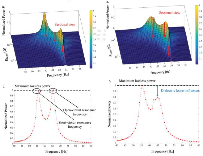
**Fig. 14.** Experimental harvested power (a) in the  $(R_{\text{load}}, f)$  plane and (b) as a function of the frequency f with an optimal  $R_{\text{load}}$  maximizing the harvested power, with  $\tan(\delta) \approx 0.1\%$  and  $\gamma = 0.01$  G.
