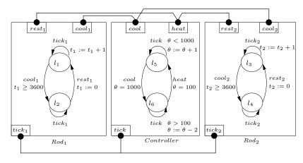
Fig. 7: Temperature Control System in BIP
