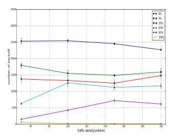
Figure 5: Number of backoffs for different rates of equipped vehicles at different densities, Thr = 1 m,  $det_r = 40 \text{ m}$
