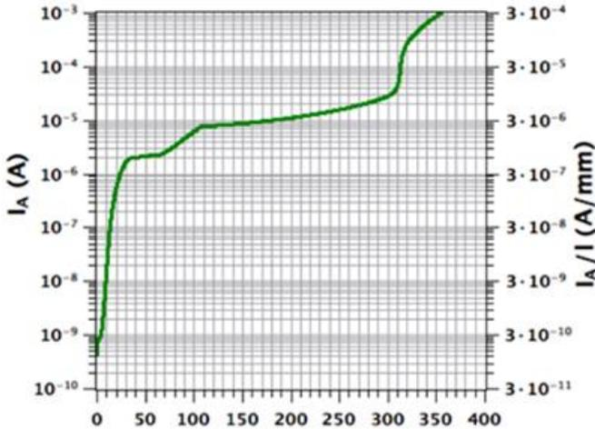
Fig. 7. Experimental static characteristic  $I_A=f(V_{AK})$  in reverse conduction for a rectifier Schottky diode with a width junction of 3.34 mm
