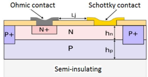
Fig. 4. Cross view of the lateral Schottky Diode. A and K represent the anode and the cathode.  $h_n$  is the thickness of the layer N.  $h_p$  is the thickness of the layer P.  $L_j$  is the length of the junction.
