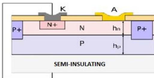
Fig. 13. Principle for the configuration C3, which has been used for the reverse conduction of the power diode. The anode (C) is connected to the metallization of the backside.
