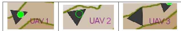
Figure 3: Representations of the three levels of searching autonomy capability; (a) UAV 1 : Fully autonomous - auto identification and selection of the Items of Interest (IOIs), (b) UAV 3 : Partially autonomous - auto identification, manual selection of the IOIs, and (c) UAV 2 : No autonomy - Manual identification and selection of the IOIs.
