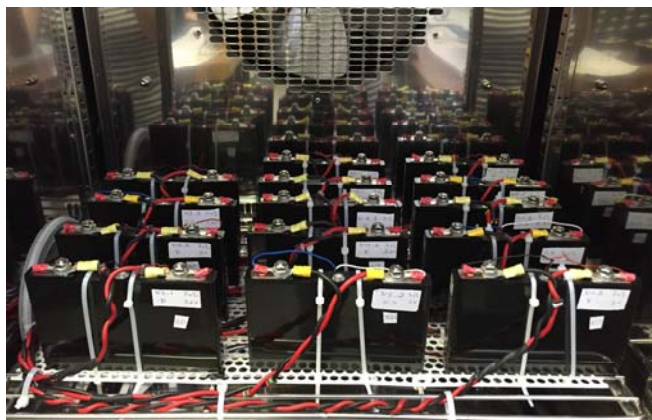
Fig. 2. LiCs mounted in a climatic chamber.
