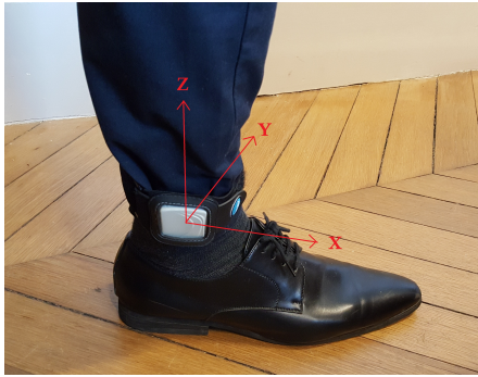
Fig. 2: Body frame definition.
