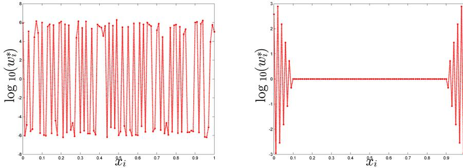
Figure 3.1: BLUE weights  $(w_i^*/|w_i^*|) \log_{10}(\max\{|w_i^*|, 1\})$  for  $x_i = (i - 1)/(n - 1)$ ,  $i = 1, \dots, n = 101$ . Left:  $K(x, x') = \exp(-|x - x'|^2)$ , Right:  $K(x, x') = (1 + \sqrt{5}|x - x'| + 5|x - x'|^2/3) \exp(-\sqrt{5}|x - x'|)$  (Matérn 5/2).
