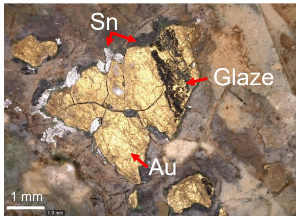
Figure 9: Micro-photography of a gold leaf from a thistle in the upper parts of room dn showing traces of a black glaze or paint layer © Piqué.
