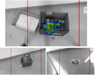
Fig. 2. On the top: uranyl acetate bottles. On the bottom left: plutonium source. On the bottom right: natural uranium bar. Detection duration and sources activities are voluntarily not stated.
