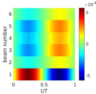
**(b)** Nonlinear time evolution of the transversal DOF at the middle of each beam (●)
