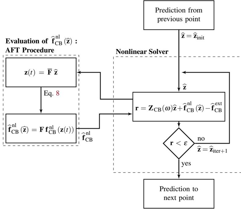
Figure 1. HBM procedure of the reduced system
