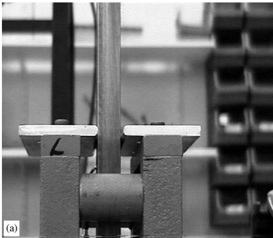
Fig. 3. Impacting beam: (a) experimental fixture; (b) measured restoring force.
