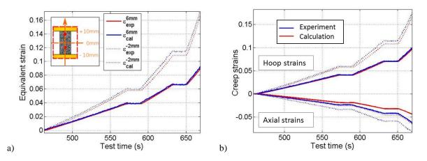
**FIGURE 6.** The experimental and calculation data are compared in this figure. Equivalent creep strains are plotted over time in a) for two different axial positions (z=-2mm for the dot lines, and z=6mm for the solid ones). Axial and hoop strains are plotted over time in b) for the same axial positions.
