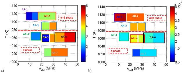
FIGURE 7. Determined a) stress exponent and b) activation energies (*J/mol*) are plotted over stresses and temperatures.
