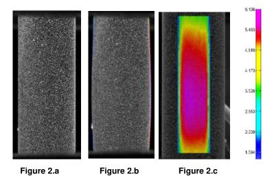
Based on the reference image (2.a) the contours are determined (2.b) and the DIC can correlate up to 13% of hoop strain (2.c) at 800°C with a good agreement
