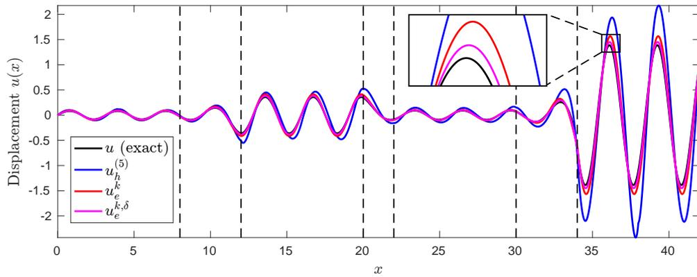
Figure 13: Exact displacement and FE approximations in the multidomain bar for  $k = 2$ . There are two elements in each straight subdomain, and one in each connection (for a total of  $N = 11$  elements), so that  $h = \max_n h_n = 4$  and the resolution is  $\lambda/h \approx 0.8$ .
