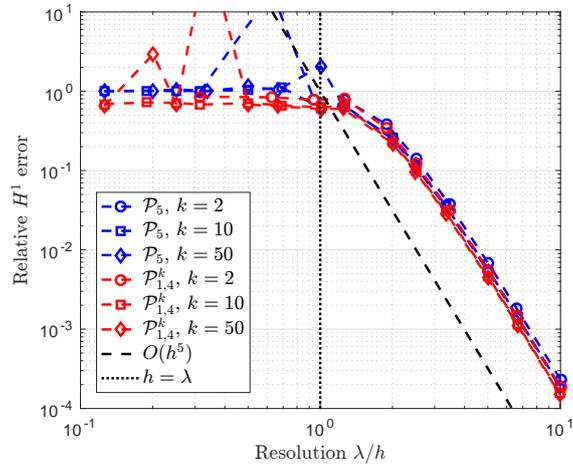
Figure 8: Convergence of solutions using the polynomial space  $\mathcal{P}_5$  (blue) and the enriched space  $\mathcal{P}_{1,4}^k$  (red), for several wavenumbers, when an oscillating force density is applied.
