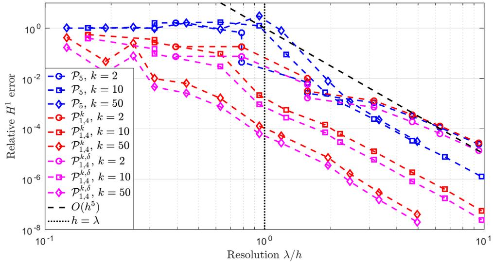
Figure 14:  $H^1$  relative errors for the multidomain bar and for polynomial (blue), sine-enriched (red) and exponential-enriched (magenta) FE spaces, and several wavenumbers.
