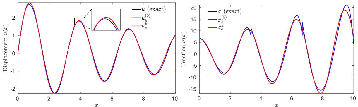
Figure 4: Exact and approximated solutions for the displacement (left) and the traction (right) in a bar with quadratic profile for  $k = 2$  and  $N = 3$  elements: the resolution is  $\lambda/h \approx 0.94$ . In both cases, the sine-enriched solution  $u_e^k$  (red) is superposed with the exact one (black).
