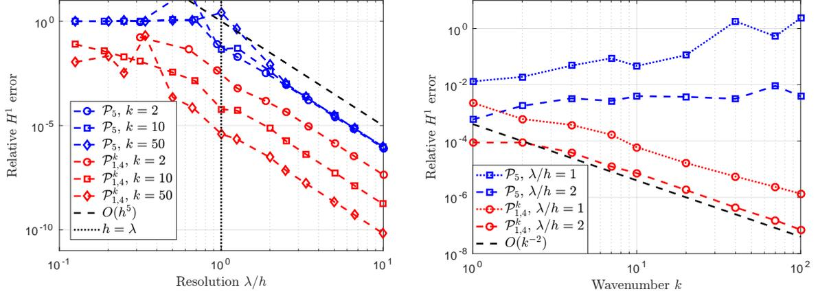
Figure 5: Relative  $H^1$  errors obtained using the polynomial space  $\mathcal{P}_5$  (blue) and the enriched space  $\mathcal{P}_{1,4}^k$  (red). Left: fixed wavenumbers  $k$  and varying resolution  $\lambda/h$ , and right: fixed resolutions  $\lambda/h$  and varying wavenumber.
