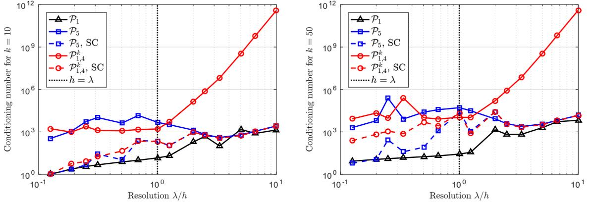
Figure 6: Conditioning number of the system to be solved, obtained without (solid lines) and with (dashed lines) static condensation, for  $k = 10$  (left) and  $k = 50$  (right). For comparison purposes, the conditioning of the matrices obtained with the space  $\mathcal{P}_1$  of linear-by-part elements is also plotted (solid black line).
