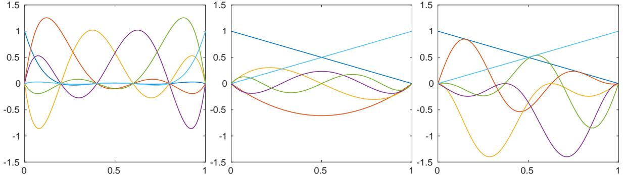
Figure 2: Basis functions on an element of length  $h = 1$ . From left to right, nodal basis of Lagrange polynomials (here with regularly spaced inner nodes), hierarchical basis of Lobatto polynomials, and sine-enriched basis  $\mathbb{P}_{1,4}^k$  for  $k = 10$ .
