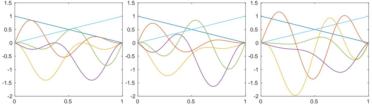
Figure 9: Shape functions of the exponential-enriched basis  $\mathbb{P}_{1,4}^{k,\delta}$  on an element of length  $h = 1$  and for  $k = 10$ . From left to right,  $\delta = 0$  (sine-enriched basis),  $\delta = 1$  and  $\delta = -2$ .
