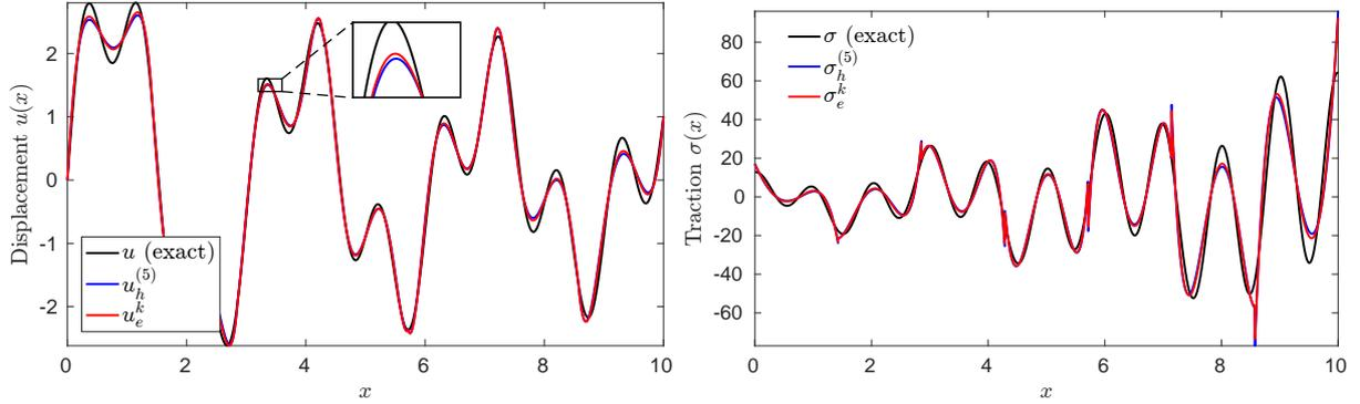
Figure 7: Exact and approximated solutions for the displacement (left) and the traction (right) in a bar with quadratic profile for  $k = 2$ , an oscillating density of forces with  $k_p = \pi k$  and  $N = 7$  elements. The resolution is  $\lambda/h \approx 2.2$ .
