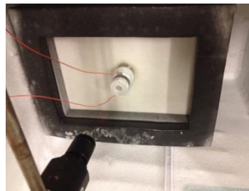
Figure 14 – Study case: bolt-clamped Langevin transducer connected to the plate
