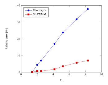
Figure 10: Impact of the aspect ratio on estimation precision of Minkowycz and SLAWMM methods
