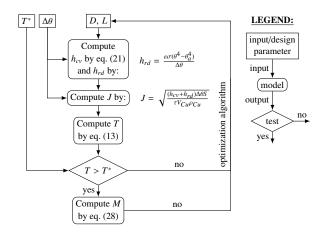
Figure 14: Preliminary LATM sizing by optimization and using the constructed metamodels. In the optimization problem,  $T > T^*$  represents the inequality constraint and the eq. (28) represents the objective function to be minimized
