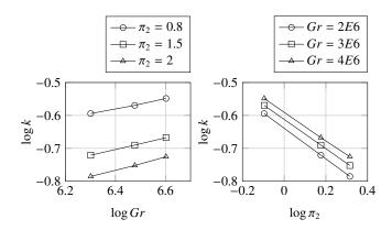
Figure 8: Plots in logarithmic bases of the multiplicative function k versus Grashof number (left) and form factor  $(\pi_2)$  (right)
