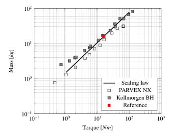
Figure 3: Brushless motor masses according to the nominal torque [26, 27]. The reference point corresponds to the motor whose data where used in the scaling law (eq. (9)) to evaluate the constant  $k_5$ .
