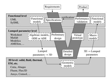
Figure 2: V-cycle diagram for the design of a mechatronic system and its associated modeling
