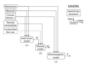
Figure 5: N-squared diagram of the LATM modeling process
