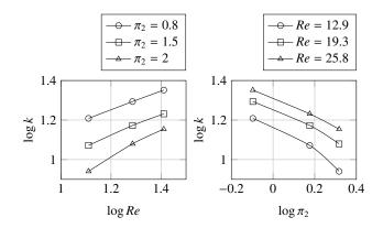
Figure 12: Plots in logarithmic bases of the multiplicative function k versus Reynolds number (left) and form factor  $(\pi_2)$  (right)
