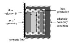
Figure 11: Simulation model for the LATM in the case of internal cooling
