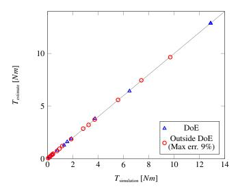
Figure 7: Comparison of the electromagnetic torques obtained by Comsol simulation,  $T_{simulation}$  and eq. (13),  $T_{estimate}$
