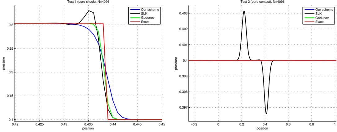
FIG. 3. Final state for Test 1 (left) and Test 2 (right) with the scheme (17)-(20) (blue), the *SLK* scheme (black), the Godunov method (green) and the exact solution (red). The mesh size is  $h = 8/4096$ .
