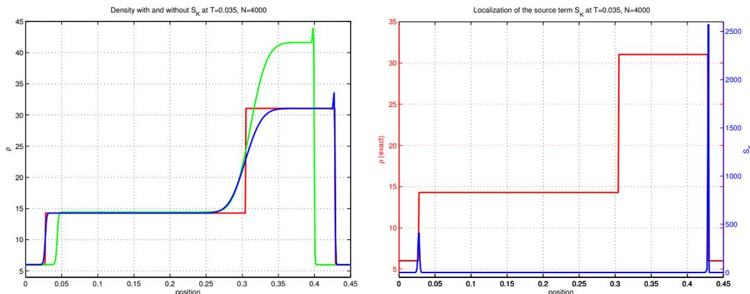
FIG. 4. Influence of the source term for Test 7. Left: density at  $T = 0.035$  with  $S_K$  (blue), without  $S_K$  (green) and exact solution (red). Right: localization of  $S_K$  (blue) with respect to the exact solution (red).
