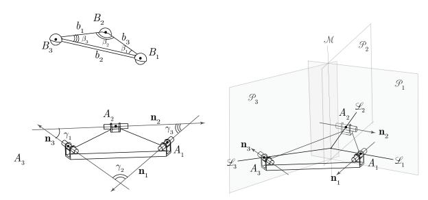
Figure 3: Similarity condition between the moving platform triangle and the triangle enclosed by the R-joint axes.
