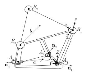
Figure 6: A 3-RPS parallel manipulator with  $n_{13} = 0$
