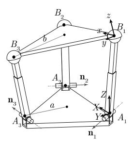
Figure 5: A 3-RPS parallel manipulator with  $n_{23} = 0$
