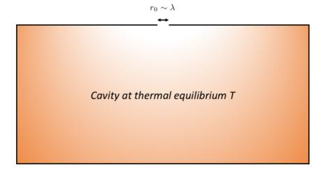
FIG. 1: Cavity at thermal equilibrium at temperature T separated from the outside by an aperture of radius  $r_0$ .
