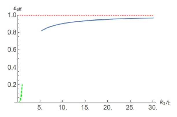
FIG. 2: Emissivity of the cavity versus  $k_0r_0$  calculated by means of fluctuation electrodynamics in the Bethe-Bouwkamp regime ( $k_0r_0 \ll 1$ , dashed-green curve) and in the Kirchhoff regime ( $k_0r_0 > 6$ , blue curve).
