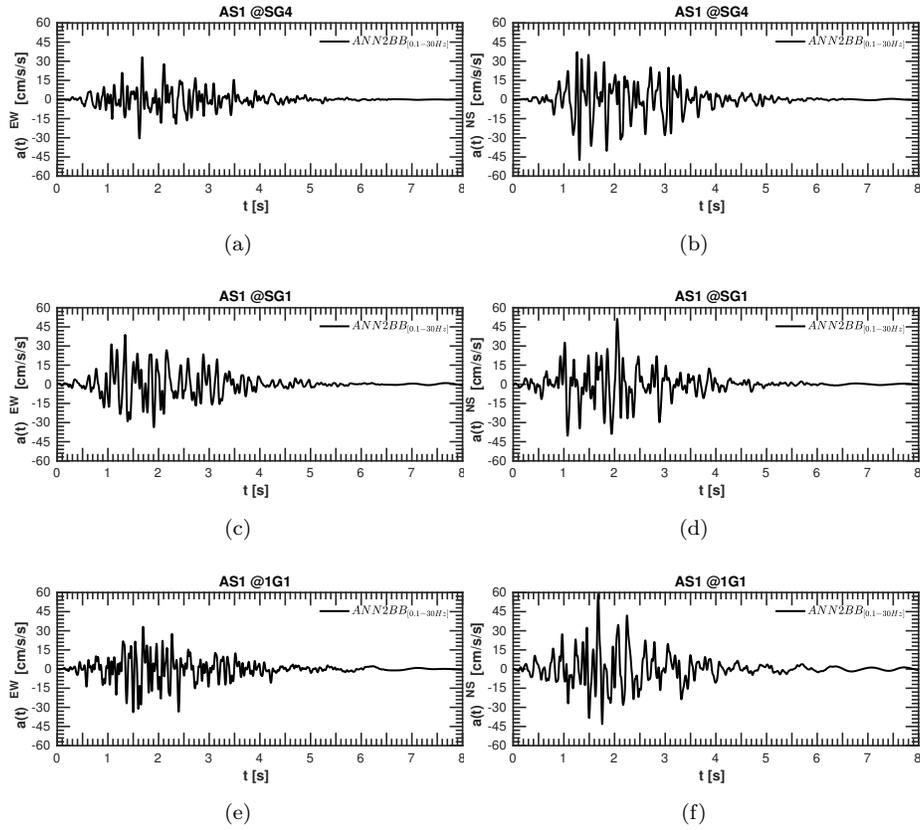
Figure 12: Acceleration time histories (EW-NS directions, in  $\text{cm/s}^2$ ) after ANN2BB application on the SEM3D analysis performed for AS1, at the Service Hall of the KKNPP site: (a-b) SG4, Service Hall, G.L. -250 m; (c-d) SG1, Service Hall, G.L. 0 m; (e-f) 1G1, Unit 1, G.L. 0 m. Synthetics were filtered between 0.1-30 Hz.
