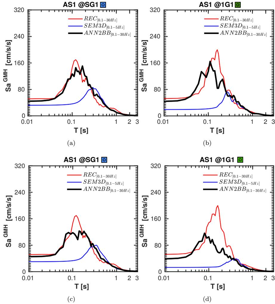
Figure 11: Pseudo-spectral acceleration response ( $Sa$ , in  $\text{cm/s}^2$ ) after ANN2BB application on the SEM3D analysis performed for AS1, at the Service Hall of the KKNPP site: (a-c) SG1, G.L. -250 m, (b-d) 1G1, G.L. 0 m respectively. REC (red), SEM3D (blue) and ANN2BB (black) are the recorded, simulated and enriched  $Sa$  spectra respectively. Synthetics labelled as REC and ANN2BB were filtered between 0.1-30 Hz, whereas SEM3D synthetics between 0.1-5 Hz.
