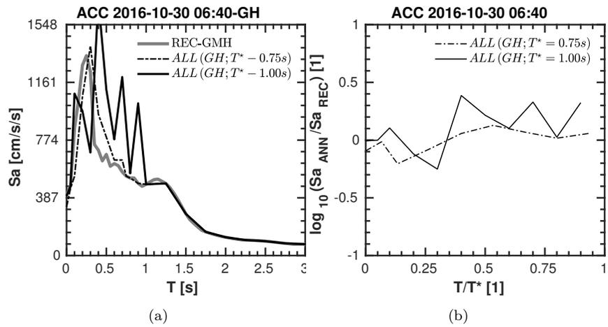
Figure 10: (a) Recorded (thick gray line) and estimated  $Sa$  spectra (geometric mean of the horizontal components), for  $T^*=0.75$  s (dashed black line) and  $T^*=1$  s (solid black line). (b) ANN performance for different training corner periods  $T^*$  (0.75 and 1 s respectively), expressed in terms of estimated/target  $Sa$ . The data refer to stations ACC, which recorded the CIT2016
