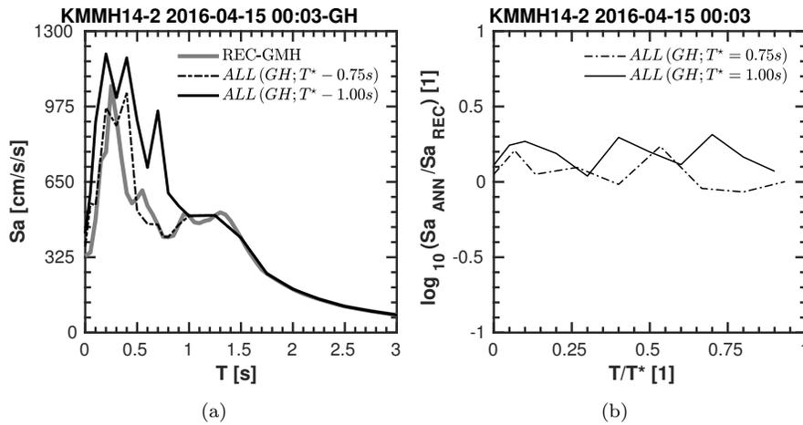
Figure 9: (a) Recorded (thick gray line) and estimated  $S_a$  spectra (geometric mean of the horizontal components), for  $T^*=0.75$  s (dashed black line) and  $T^*=1$  s (solid black line). (b) ANN performance for different training corner periods  $T^*$  (0.75 and 1 s respectively), expressed in terms of estimated/target  $S_a$ . The data refer to station KMMH14, which recorded the KMM2016
