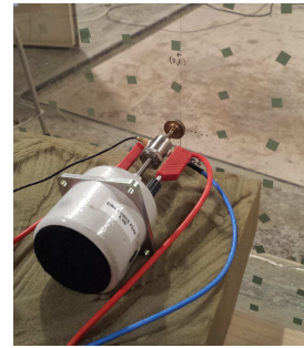
Figure 3: Shaker test set up of the single layer glass plate of size 0.012 x 1.35 x 1.54 m.
