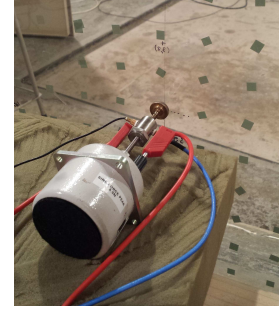
Figure 3: Shaker test set up of the single layer glass plate of size 0.012 \times 1.35 \times 1.54 m.
