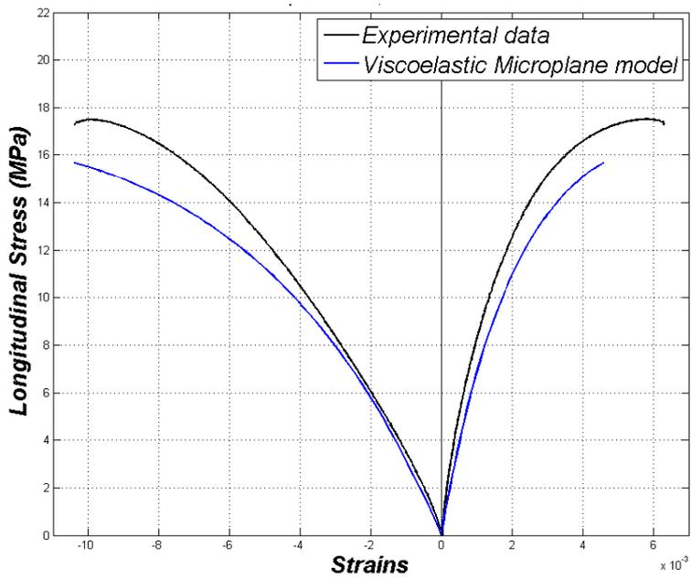
Figure 11. Experimental and numerical  $\sigma$ - $\epsilon$  curves of monotonic compression test, strain rate =  $4.4 \times 10^{-6}/s$
