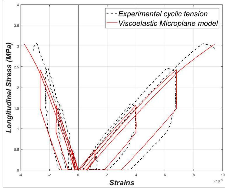
Figure 6. Experimental and numerical  $\sigma$ - $\epsilon$  curves of cyclic tension results
