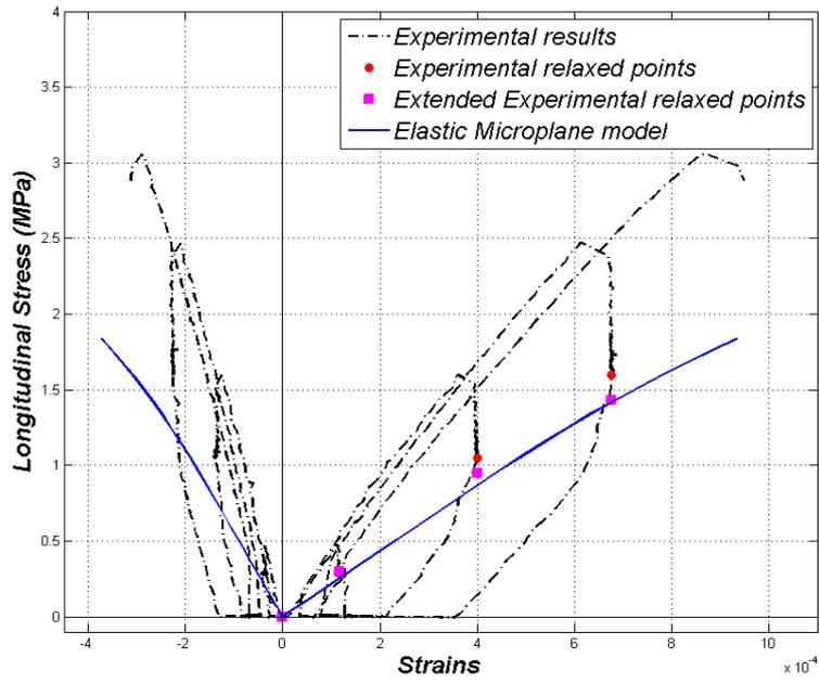
Figure 4. Calibrating damage parameters based on extended experimental relaxed points of cyclic tension
