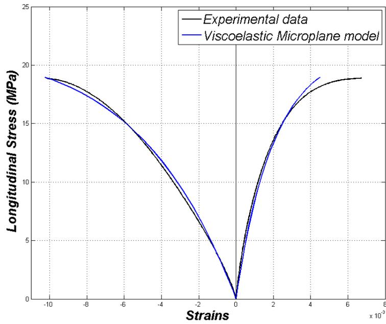
Figure 10. Experimental and numerical  $\sigma$ - $\epsilon$  curves of monotonic compression test, strain rate =  $3.3 \times 10^{-5}/s$
