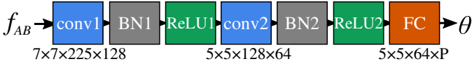
Fig. 4. Architecture of the regression network. It is composed of two convolutional layers without padding and stride equal to 1, followed by batch normalization and ReLU, and a final fully connected layer which regresses to the P transformation parameters.
